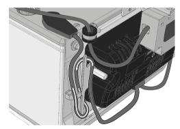
Figure 183. Attach the cable that is connected to the rear battery's left terminal on its cable holder as shown.
