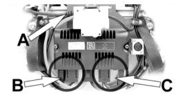
Figure 178. Connectors (B) and (C); for disconnection.
