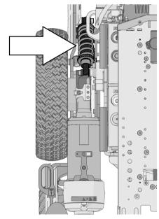
Figure 4. Drive unit and shock absorber.
