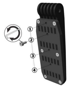
Figure 40. Height adjustment screw.
