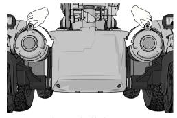
Figure 137. Releasing wheel lock.
