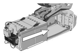
Figure 185. Push in the battery box.
