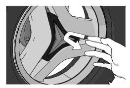
Figure 154. Use your fingers as follows on two edges of the hub cap.
