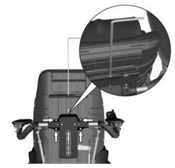
Figure 25. Adjusting the armrest height.
