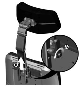
Figure 39. Removal of headrest.
