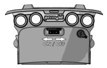
Figure 8. Main circuit breaker location.
