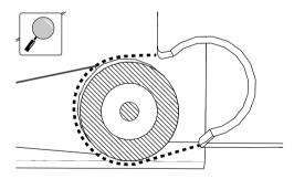
Figure 176. An enlargement of the rear cover going over the rear axle.
