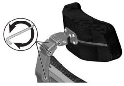
Figure 41. Adjust height and depth.
