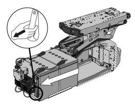
Figure 179. Straps for pulling out battery box.
