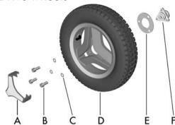
Figure 149. Assembly of the drive wheel.
