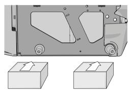
Figure 164. Use two blocks on each side of the chassis box. The wheels has been removed in this figure for better viewing.
