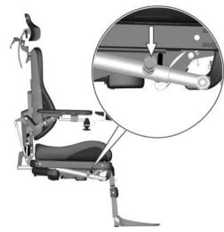
Figure 17. Manually adjusting leg rest angle.
