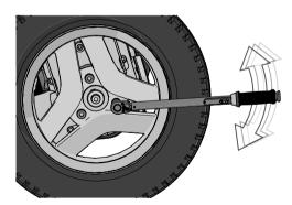
Figure 157. Use a torque wrench to tighten the screws.
