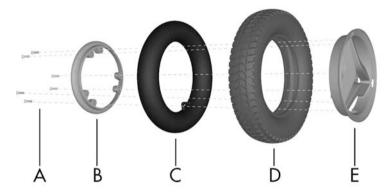
Figure 159. Assembling a pneumatic tire to a split rim.
