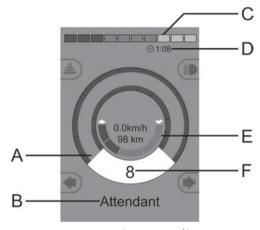
Figure 54. Drive screen when set to profile 8.
