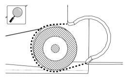
Figure 189. An enlargement of the rear cover going over the rear axle.
