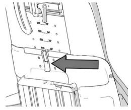
Figure 28. Clip holding the backrest.
