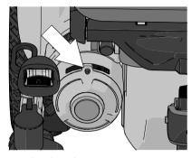
Figure 148. Brake release lever.
