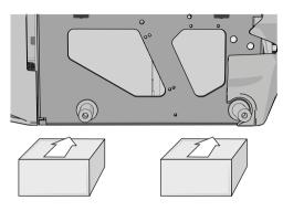
Figure 152. Use two blocks on each side of the chassis box. The wheels has been removed in this figure for better viewing.
