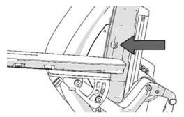
Figure 30. Trunk support screw.
