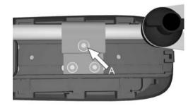
Figure 33. Screw for adjusting the panel holder length.
