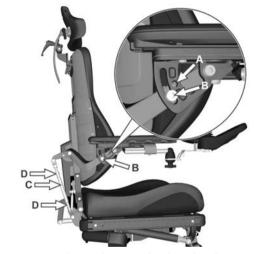
Figure 27. Adjusting the armrest height and angle.
