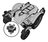
Figure 173. The chassis covers are secured with two knobs.
