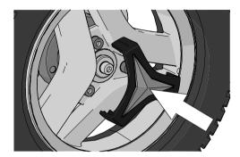
Figure 158. The hub cap snaps when it is in place.
