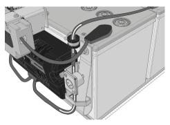
Figure 184. Attach the cable that is connected to the front battery's right terminal in its cable holder as shown.
