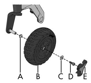
Figure 161. Assembly of rim.
