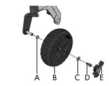
Figure 166. Assembly of rim.
