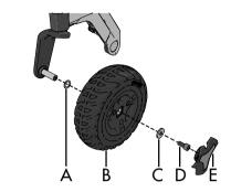
Figure 167. Assembly of rim.
