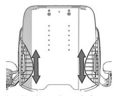
Figure 31. Adjusting trunk support height.
