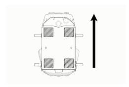
Figure 165. The position of the blocks. The arrow points in the direction of travel.
