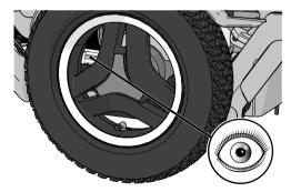
Figure 144. Chassis identification number label.
