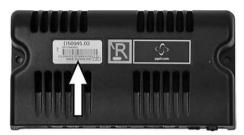
Figure 146. R-net power module ID number.
