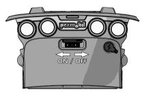
Figure 192. Main circuit breaker located under the rear lights.
