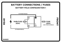
Figure 201. Battery terminals, main circuit breaker and fuse, apply to products equipped with 60 Ah batteries.
