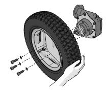
Figure 155. Pull the wheel straight out after you have removed the three screws.
