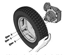
Figure 156. Mount the wheel onto the wheel hub.
