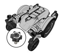
Figure 191. The chassis covers are secured with two knobs.
