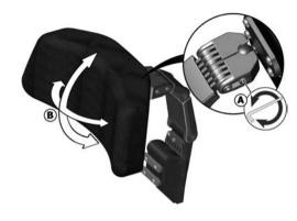
Figure 42. Adjustment of headrest angle.
