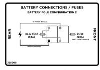
Figure 202. Battery terminals, main circuit breaker and fuse, apply to products equipped with 73 Ah batteries.
