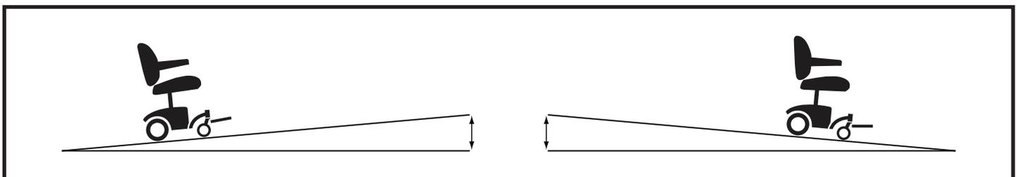
**Figure 2. Maximum Rated Slope Angle (Ascending and Descending)**
