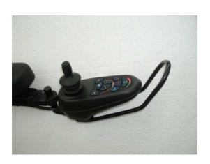
You can avoid collisions between the joystick and other objects with the joystick protection guard.
